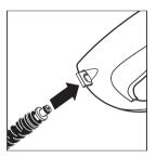
→ STEP 3: Push the locking slide back into the trigger gun (C) to lock the hose in position.
